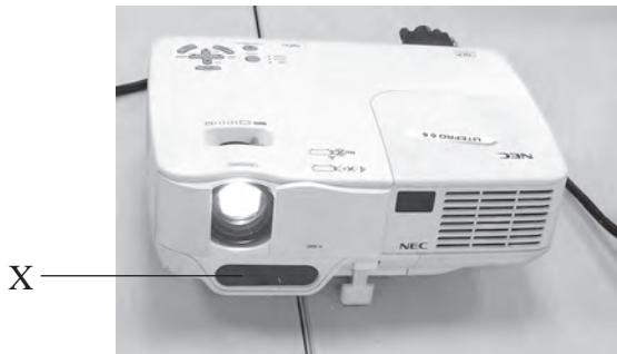
The part of the projector labelled X emits a pulse of infrared radiation and detects the pulse after it is reflected from a screen.
